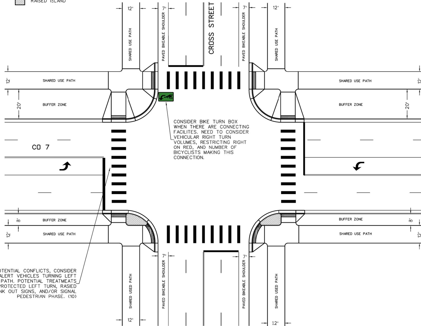
TO REDUCE POTENTIAL CONFLICTS, CONSIDER TREATMENTS TO ALERT VEHICLES TURNING LEFT OF SHARED USE PATH. POTENTIAL TREATMENTS INCLUDE SIGNAGE, PROTECTED LEFT TURN, RASIED CROSSWALK, BLANK OUT SIGNS, AND/OR SIGNAL PEDESTRIAN PHASE. (10)
