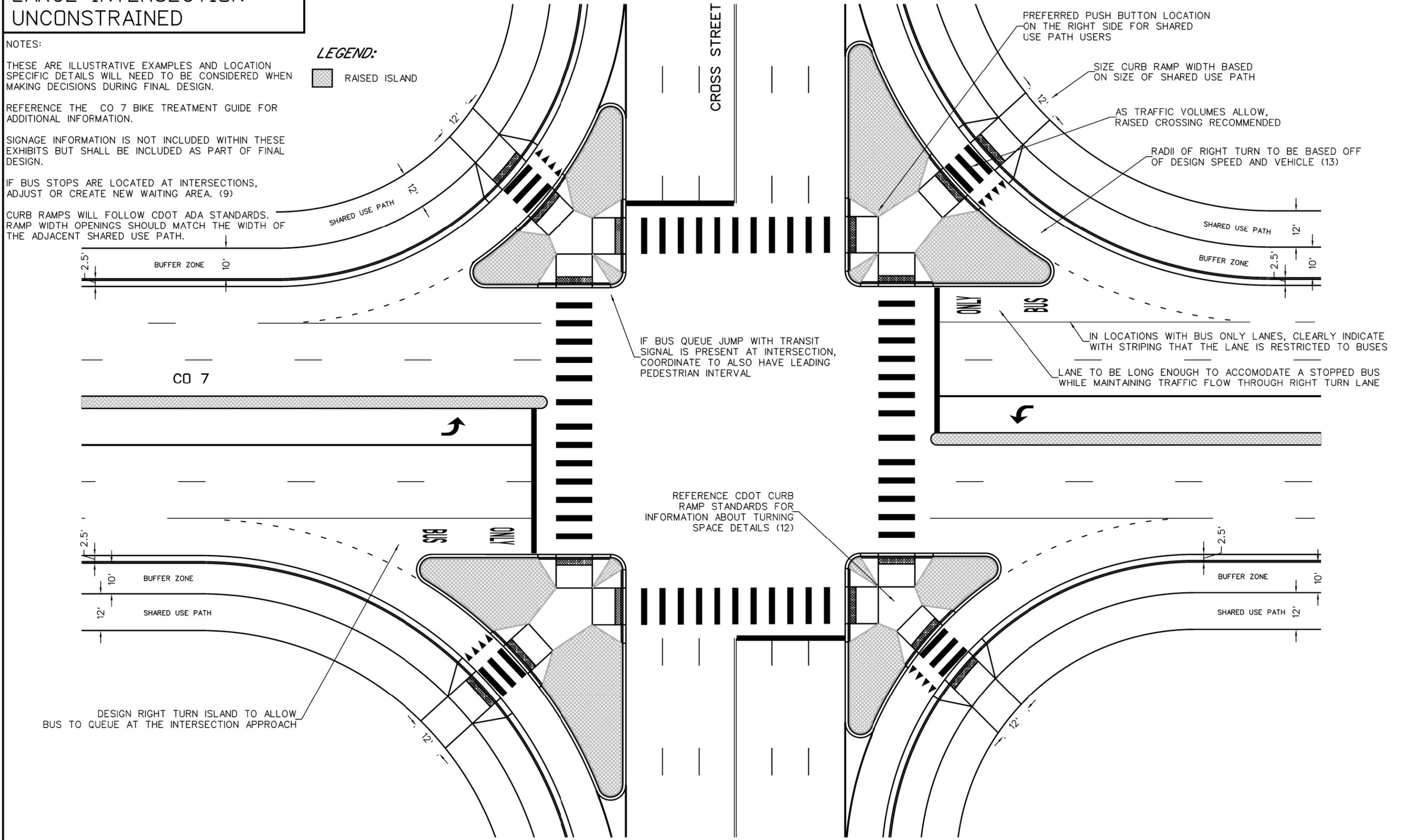
IF BUS QUEUE JUMP WITH TRANSIT SIGNAL IS PRESENT AT INTERSECTION, COORDINATE TO ALSO HAVE LEADING PEDESTRIAN INTERVAL
