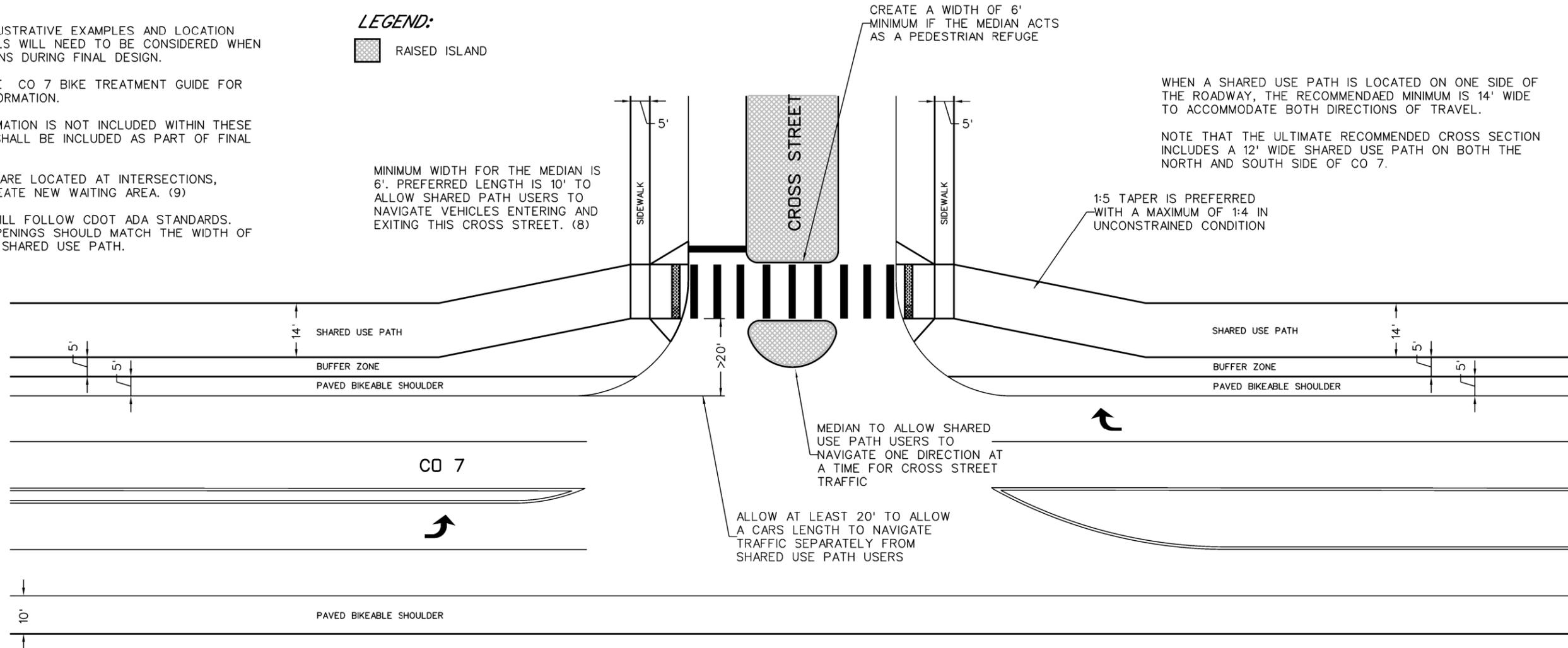
WHEN A LOCAL BUS STOP IS LOCATED AT AN INTERSECTION WITHOUT TRAFFIC CONTROL ON CO 7, CONSIDER A CROSSING. BASED ON CURRENT CDOT PEDESTRIAN CROSSING GUIDELINES, CROSSINGS SHOULD NOT BE INSTALLED ON ANY ROADWAYS THAT HAVE A POSTED SPEED LIMIT OF 45 MILES PER HOUR OR MORE. (6)
