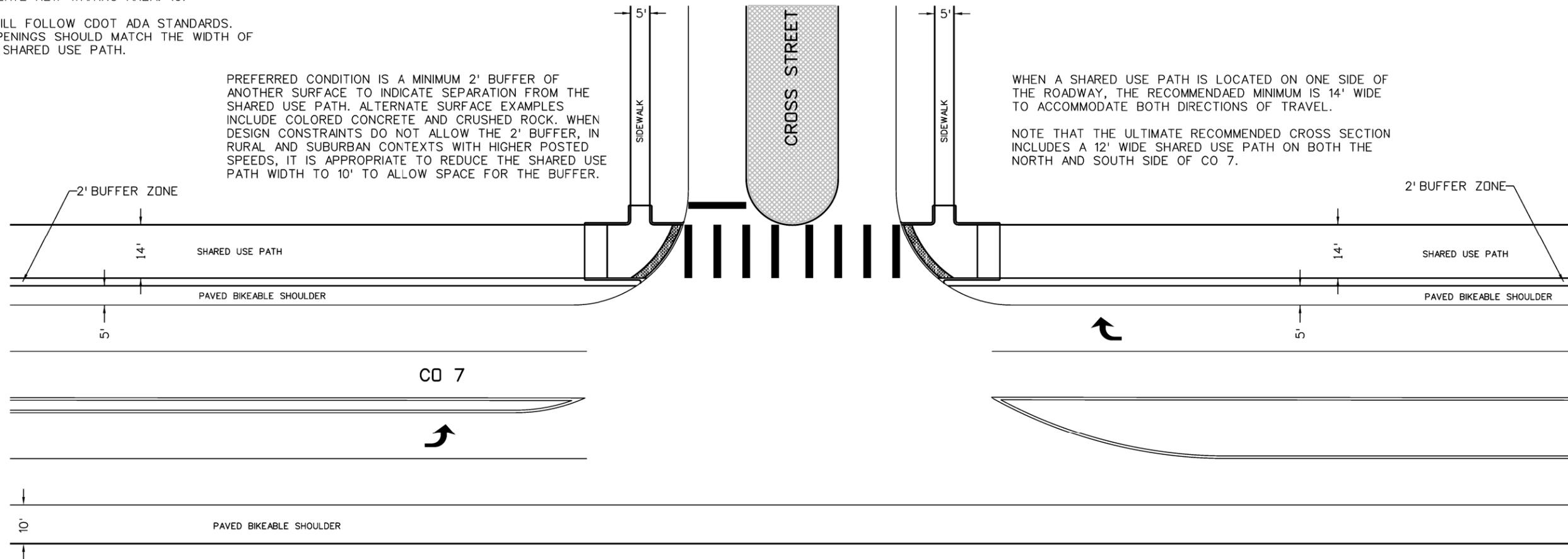
WHEN A LOCAL BUS STOP IS LOCATED AT AN INTERSECTION WITHOUT TRAFFIC CONTROL ON CO 7, CONSIDER A CROSSING. BASED ON CURRENT CDOT PEDESTRIAN CROSSING GUIDELINES, CROSSINGS SHOULD NOT BE INSTALLED ON ANY ROADWAYS THAT HAVE A POSTED SPEED LIMIT OF 45 MILES PER HOUR OR MORE. (6)
